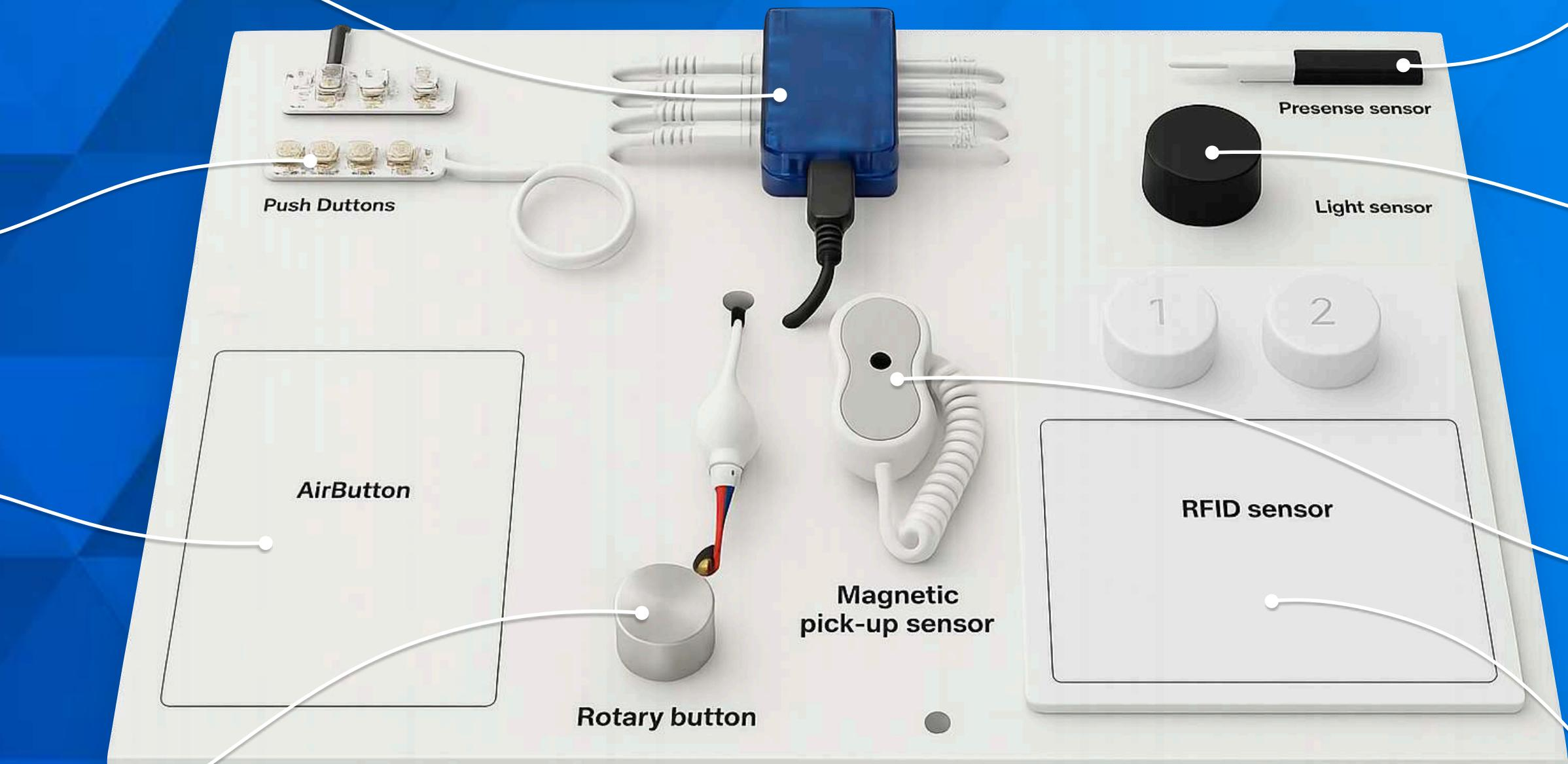
**Presence sensor** detects when a person is in front of the display, automatically activating screens, lighting, or sound.
