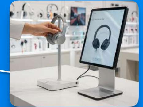
**RFID sensor** identifies objects through RFID tags, triggering specific content for each product or category when brought near the reader area.
